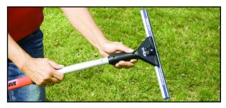
9) To use the squeegee, remove the ProCurve Tool Handle with the wash sleeve by pulling off of the pole, then attach the ProCurve squeegee.
