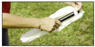
3) The ProCurve squeegee also comes fully assembled and ready to go. The 18" squeegee channel with rubber can be replaced by loosening the knob on the top of the handle and
